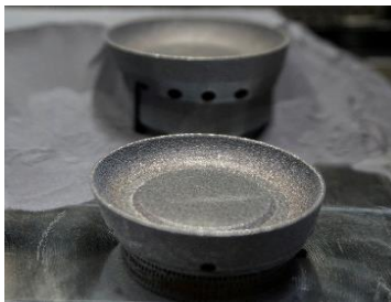
(Photos from KIEFER: manufacture of mold insert bottom)
